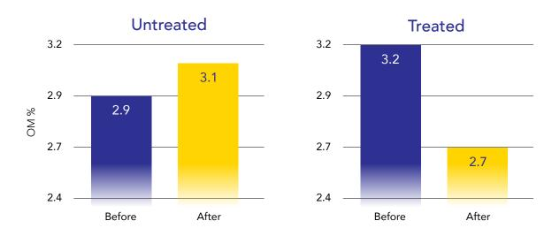
Field trial: Sand/soil push-up green. Week 1, half the green was treated with T-Thatch at 48L/Ha. 23 days later the entire green was scarified. T-Thatch was then applied monthly, 3 more times at 48L/Ha and 3 fertiliser applications were also applied. Organic matter readings week 1 and 18 show that T-Thatch consumed accumulated OM created by the growth cycle and provided lower OM compared to the untreated half of the green.
